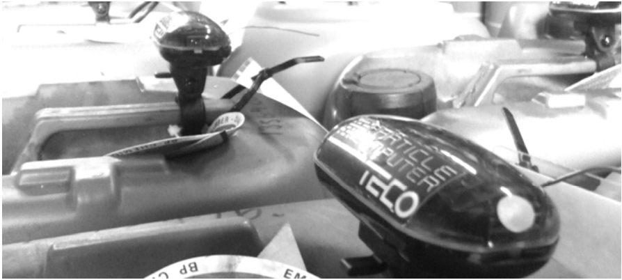
Fig. 1. Smart chemical drums equipped with sensor nodes
